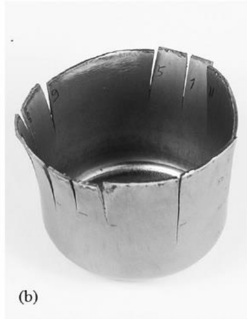
Deep drawn cups: (a) 301-2.0-S, (b) 201-2.0-S and (c) 204Cu-2.0-S. Inner diameter of the cups is 50 mm. ( Ortega et al, FFEMS 2014)
