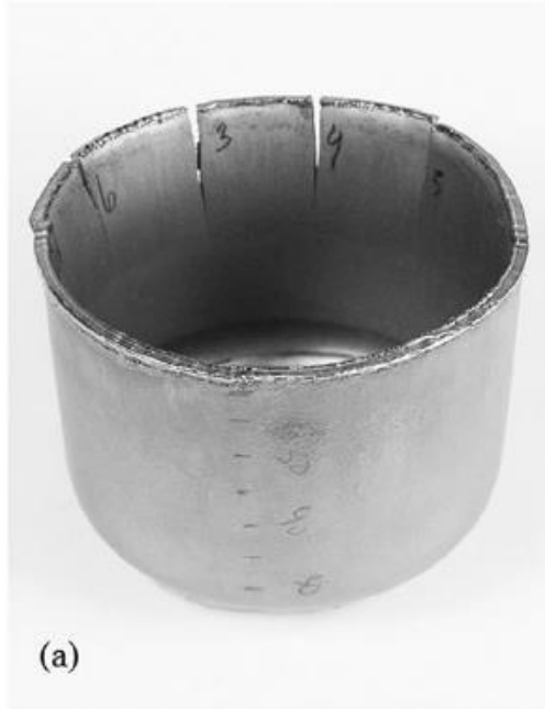
Deep drawn cups: (a) 301-2.0-S, (b) 201-2.0-S and (c) 204Cu-2.0-S. Inner diameter of the cups is 50 mm. ( Ortega et al, FFEMS 2014)
